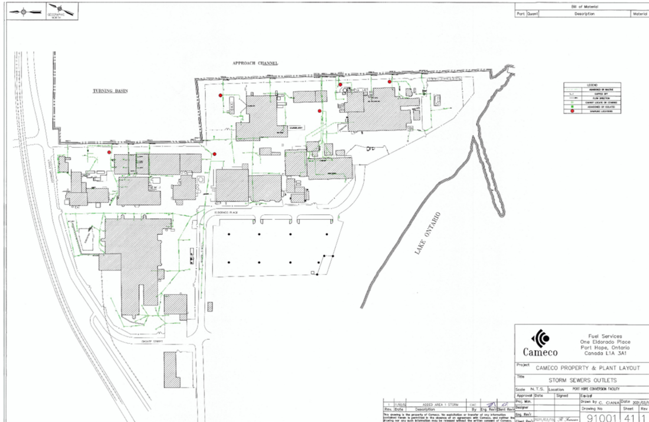
Figure 36: Storm Sewer Outlets
